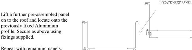
previously fixed Aluminium profile. Secure as above using fixings supplied.
