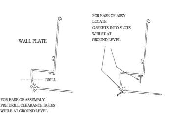
2. Secure the assembled Wall Plate to the wall using appropriate fixings (no wall fixings are supplied)
