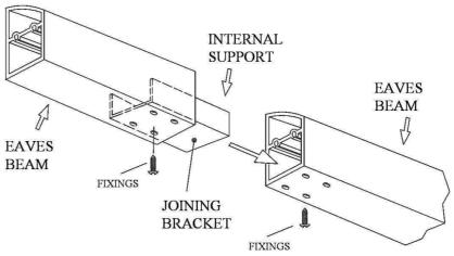
Please ensure the Eaves Beam is installed with the slope away from the wall.(See diagram)
